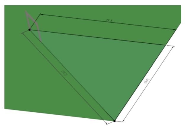
Step 8 Now we are going to place the 2 flags. From the zero walk out 24.0 m and then from the 18.3m mark walk up 15.5m. Place a flag spike. For the next flag walk out 36.2m from the zero and walk up 25.6m from the 25.6m mark. Place another flag spike.
