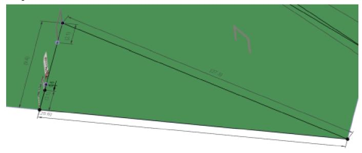
Step 7 Now take your long tape measure and go back to the 0 mark. Walk out 14.7m. Then from the 9.4m mark walk out 11.3m. Where these 2 meet, gate rebar. On the 14.7m line, also place a gate rebar at 12.6m.
