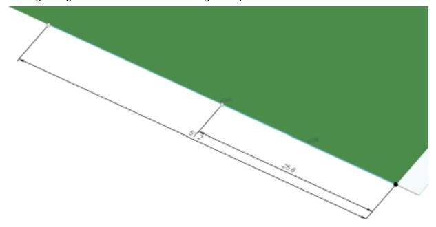
Step 3 Now we will square the track. From the 25.6m rebar walk out 36.9m. Then with the other tape measure, go to your zero and walk out 26.5m. Where these 2 meet place a marker. Also place a marker at 9.4m, a gate leg rebar at 18.3m, and a marker at 25.6m.
