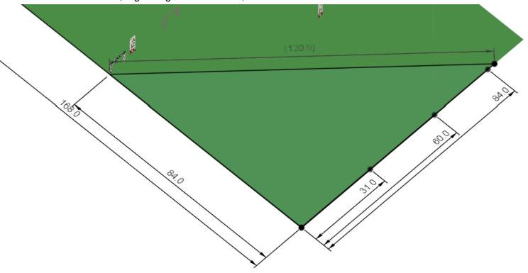
Step 4 We are now going to get the location for the 2 gates and flag. Take one tape measure and go to the 25.6m gate rebar and walk out 27.3m. Then with the other tape measure walk up 9.4m from the 51.2m mark. Where these 2 meet place a gate rebar.
